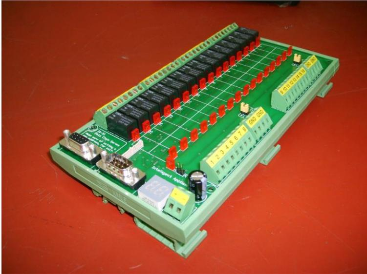
*Figure 12: IA 3126-2 relay board*
